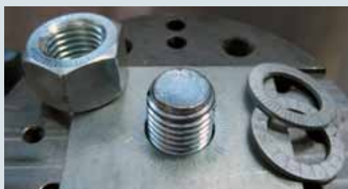
After disassembly, impression marks must be visible on both the fastener and the contact surface.
