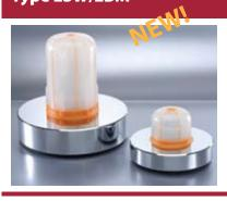
The cap is produced in a two component molding. These new caps feature a captive soft sealing lip made from Evoprene; an elastic, flexible material that can be adapted to suit the base, hence providing an excellent seal. The cap body is made from a more solid material, guaranteeing a reliable and stable hold.
